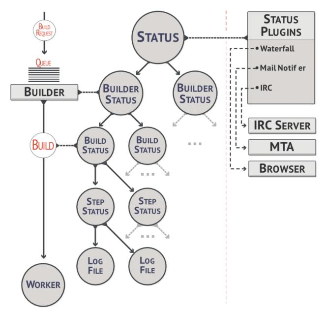
The configuration file controls which status plugins are active. Each status plugin gets a reference to the top-level Status object. From there they can request information on each Builder, Build, Step, and LogFile. This query-on-demand interface is used by the html.Waterfall plugin to create the main status page each time a web browser hits the main URL.
