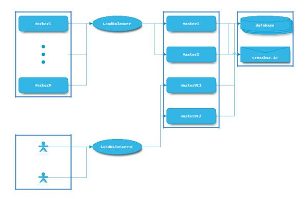
Buildbot supports interconnection of several masters. This has to be done through a multi-master enabled message queue backend. As of now the only one supported is wamp and crossbar.io. see *wamp*
